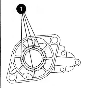
Checking commutator end shield
